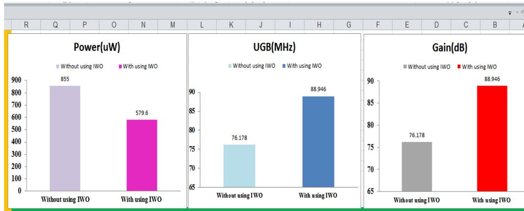
Figure .18. Comparison of the performance parameters (power, UGB, Gain) for Two Stage CMOS Op-Amp with & without using IWO.
