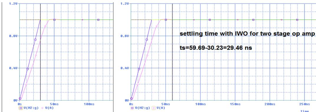
Figure .16. Simulation result of settling time measurement
