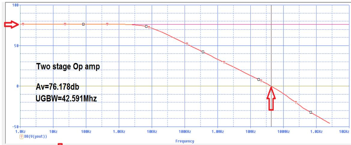
Figure 3. Simulation result (Gain measurement)
