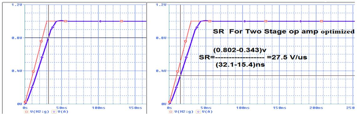
Figure .15. Simulation result of slew rate (SR) measurement
