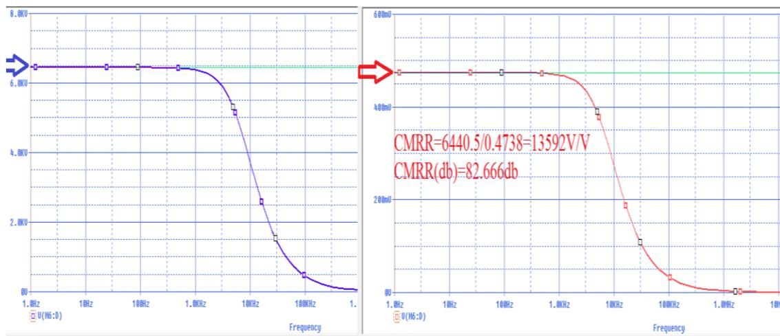
Figure .11. Simulation result of Common Mode Rejection Ratio (CMRR)
