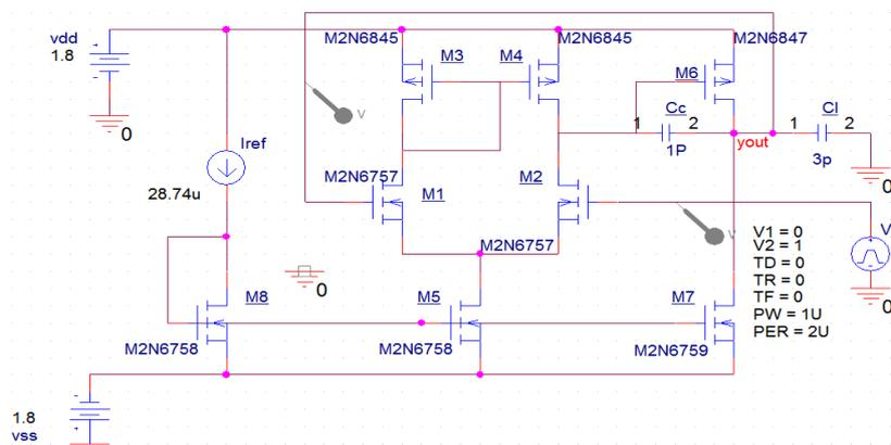
**Figure 7.** The practical circuit of two stage Op-Amp connected as a buffer used to test the value of slew rate and settling time.
