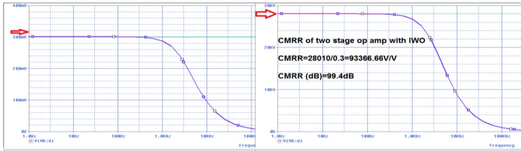
Figure .17. Simulation result of measurement Common Mode Rejection Ratio (CMRR)
