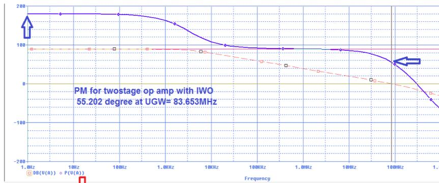
Figure .14. Simulation result of frequency response (phase measurement).
