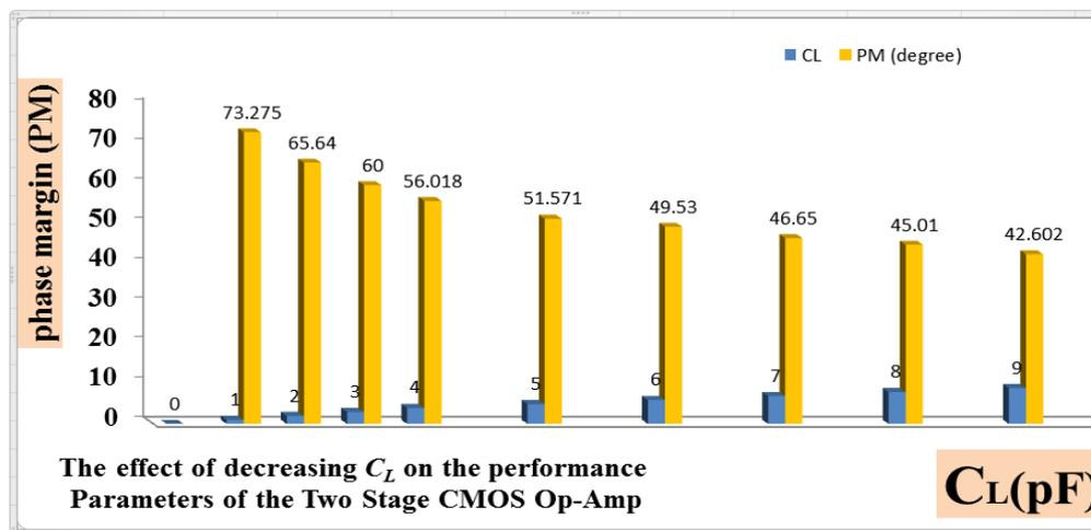
**Figure 6.** The effects of change the value of  $C_L$  on the phase margin
