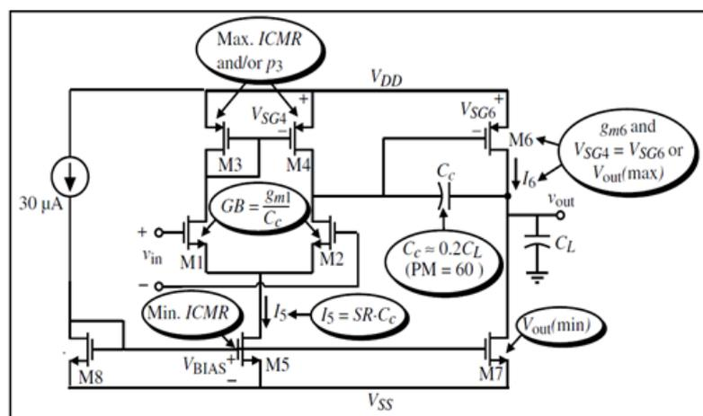
Figure. 1. Circuit& design relationship for two Stage CMOS Op-Amp.
