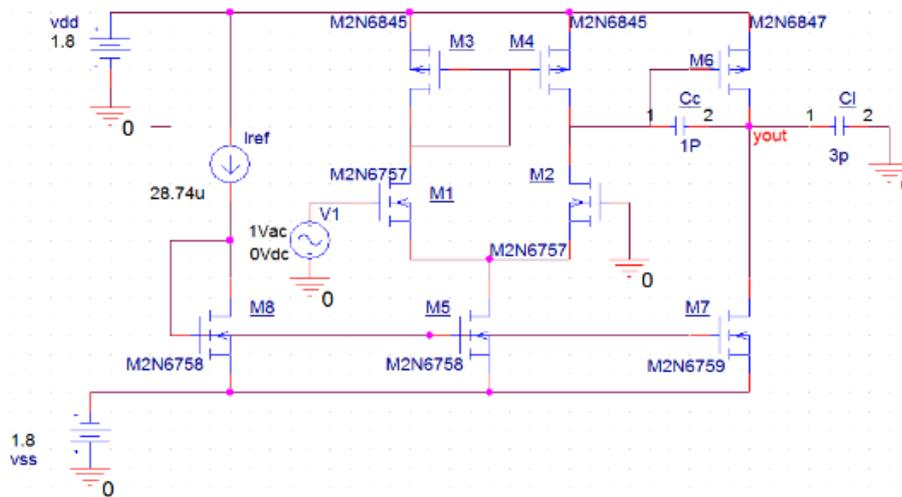
**Figure 2.** Practical circuit diagram for the Two Stage CMOS Op-Amp
