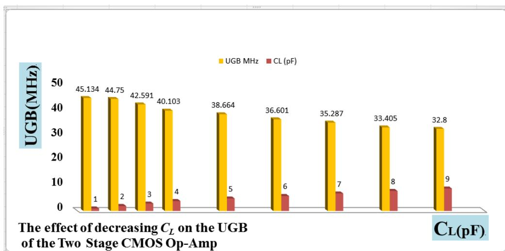
Figure 5. The effects of change the value of  $C_L$  on the UGB
