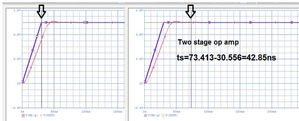
Figure 9. Simulation result of settling time ( $t_s$ ) measurement.
