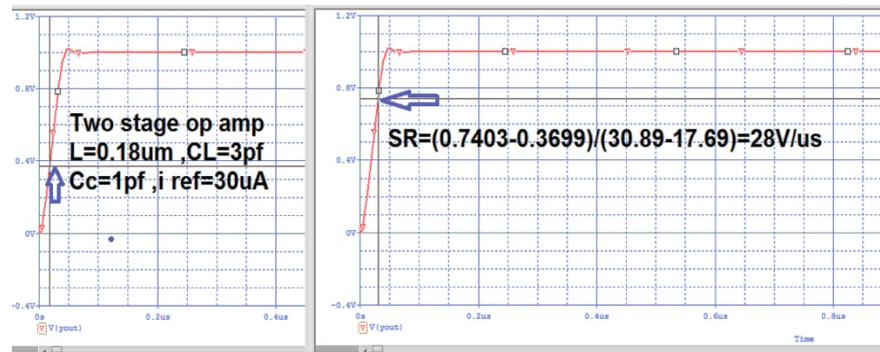
Figure 8. Simulation result of measurement of Slew Rate (SR).
