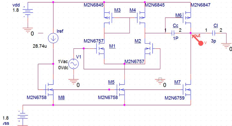
Figure .10. The practical circuit connected in common mode configuration used to calculate the value of CMRR
