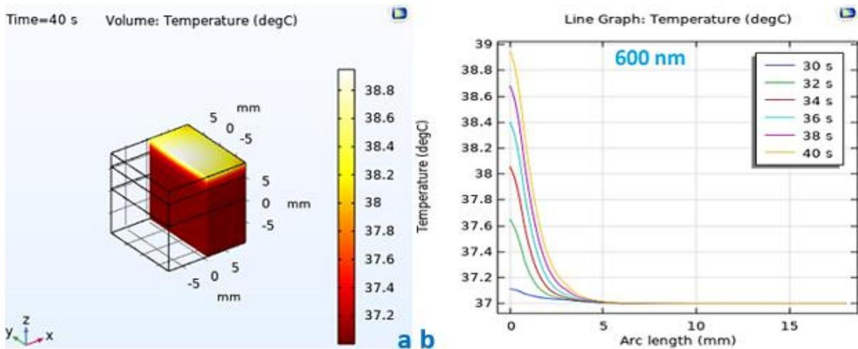
**Figure 2.** (a) 3D schematic of the temperature distribution in entire geometry, after 40 seconds in wavelength of 600 nm. (b) Line graph of the temperature distribution at several times and in different depth of sample, in wavelength of 600 nm.
