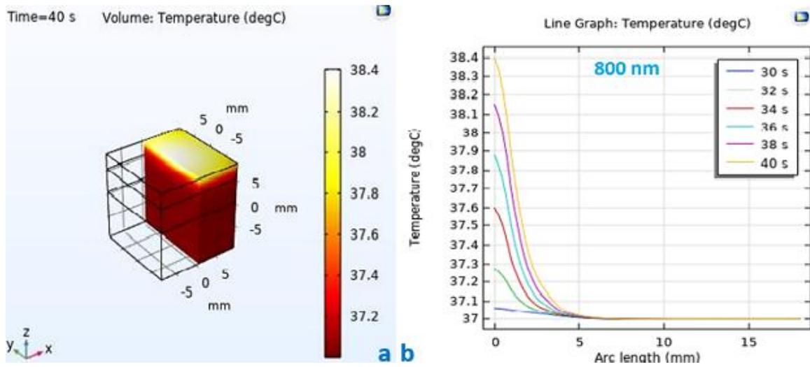
**Figure 4.** (a) 3D schematic of the temperature distribution in entire geometry, after 40 seconds in wavelength of 800 nm. (b) Line graph of the temperature distribution at several times and in different depth of sample, in wavelength of 800 nm.
