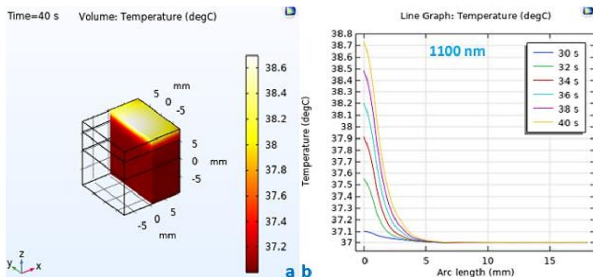
**Figure 7.** (a) 3D schematic of the temperature distribution in entire geometry, after 40 seconds in wavelength of 1100 nm. (b) Line graph of the temperature distribution at several times and in different depth of sample, in wavelength of 1100 nm.
