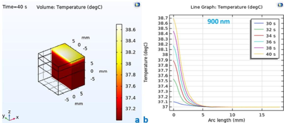
**Figure 5.** (a) 3D schematic of the temperature distribution in entire geometry, after 40 seconds in wavelength of 900 nm. (b) Line graph of the temperature distribution at several times and in different depth of sample, in wavelength of 900 nm.
