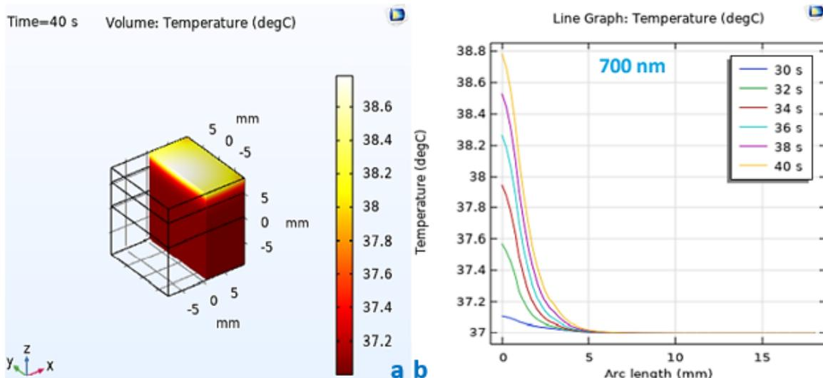
**Figure 3.** (a) 3D schematic of the temperature distribution in entire geometry, after 40 seconds in wavelength of 700 nm. (b) Line graph of the temperature distribution at several times and in different depth of sample, in wavelength of 700 nm.
