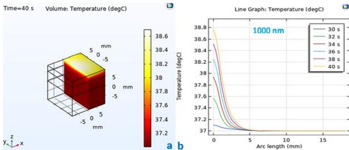
**Figure 6.** (a) 3D schematic of the temperature distribution in entire geometry, after 40 seconds in wavelength of 1000 nm. (b) Line graph of the temperature distribution at several times and in different depth of sample, in wavelength of 1000 nm.
