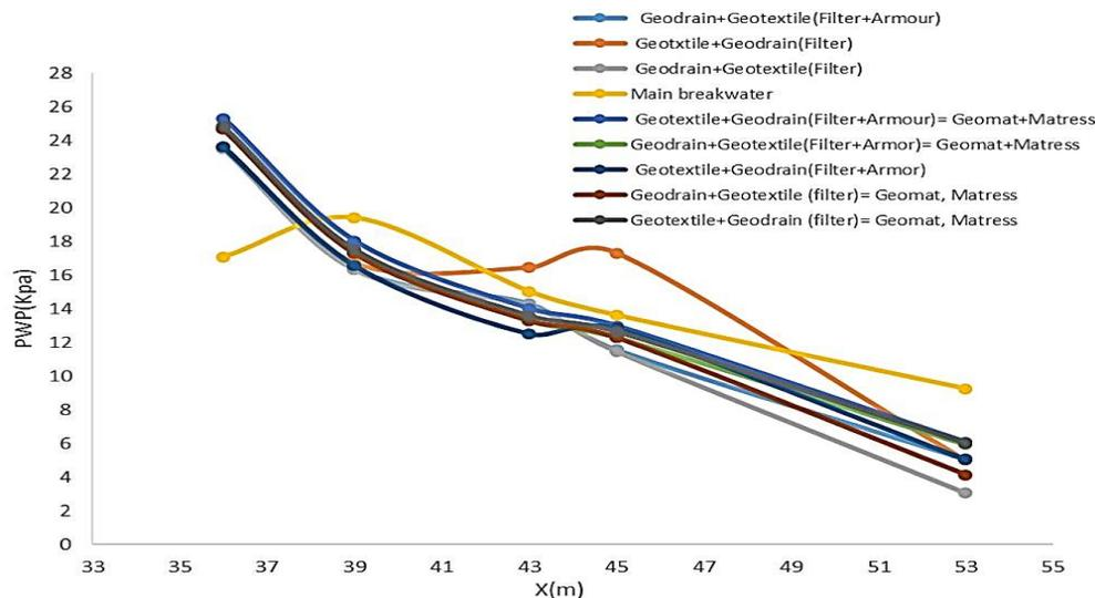
Figure 22. Comparison of pore pressure curve in all models
