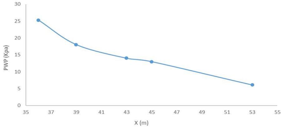
**Figure 21.** The pore pressure curve when using geodrain and geotextile as filter, armor and geomat as matress
