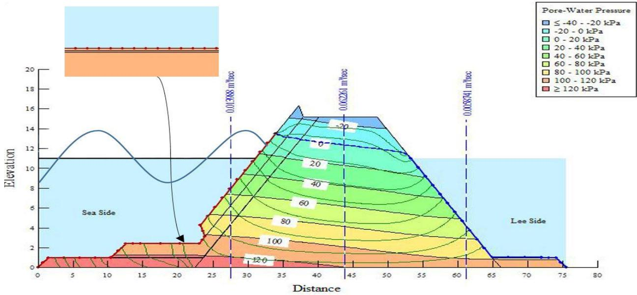
Figure 12. Use of geotextile and geodrain as filter layer and secondary armor layer
