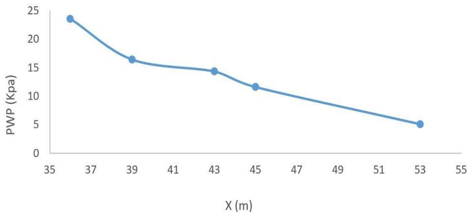
Figure 11. The pore pressure curve when using geodrain and geotextile as secondary armor and filter layer
