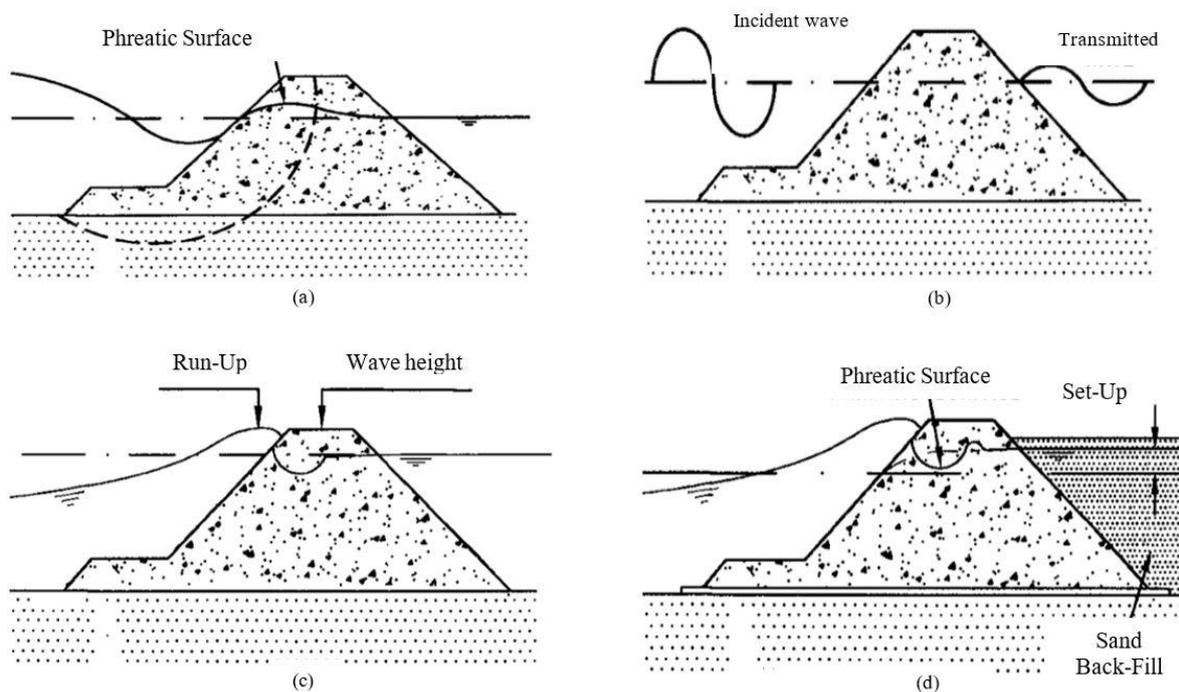
Figure 3. Different types of design under the influence of pore pressure [7].
