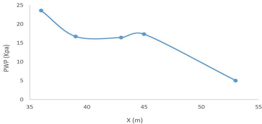
**Figure 8.** The pore pressure curve when using geotextile and geodrain
