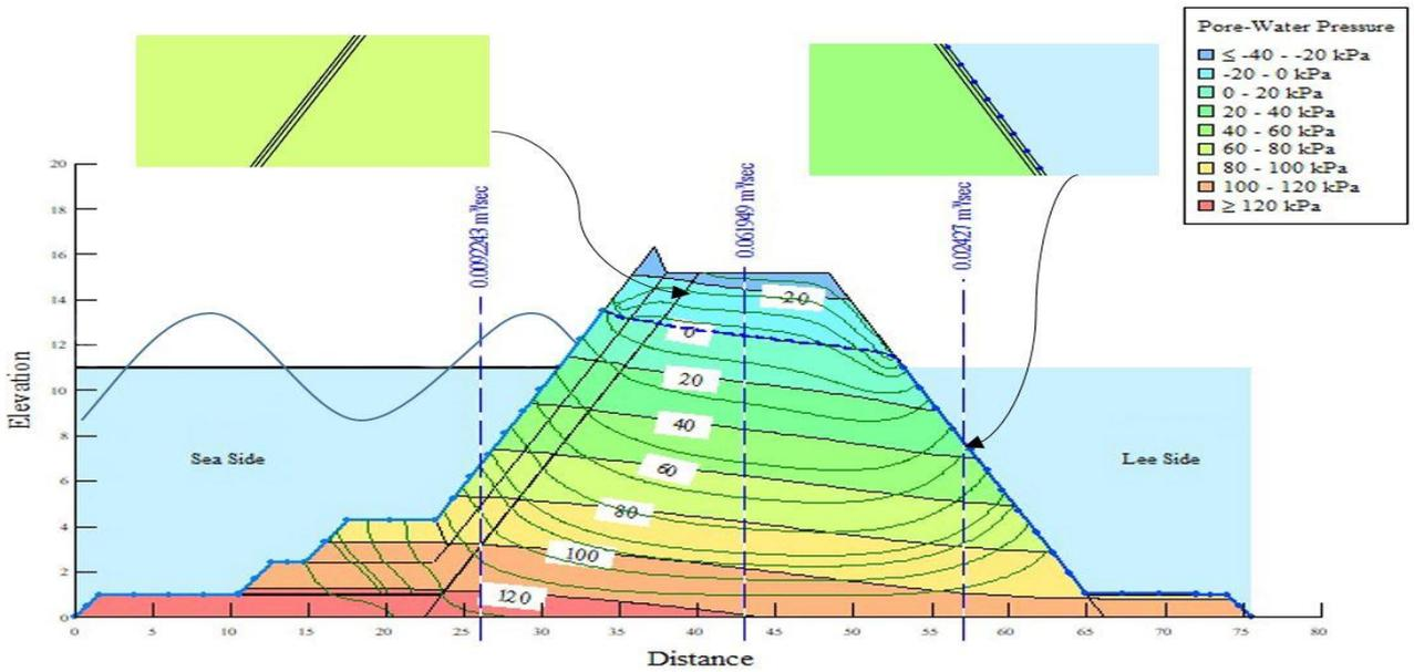
Figure 7. Use of geodrain and geotextile as filter layer
