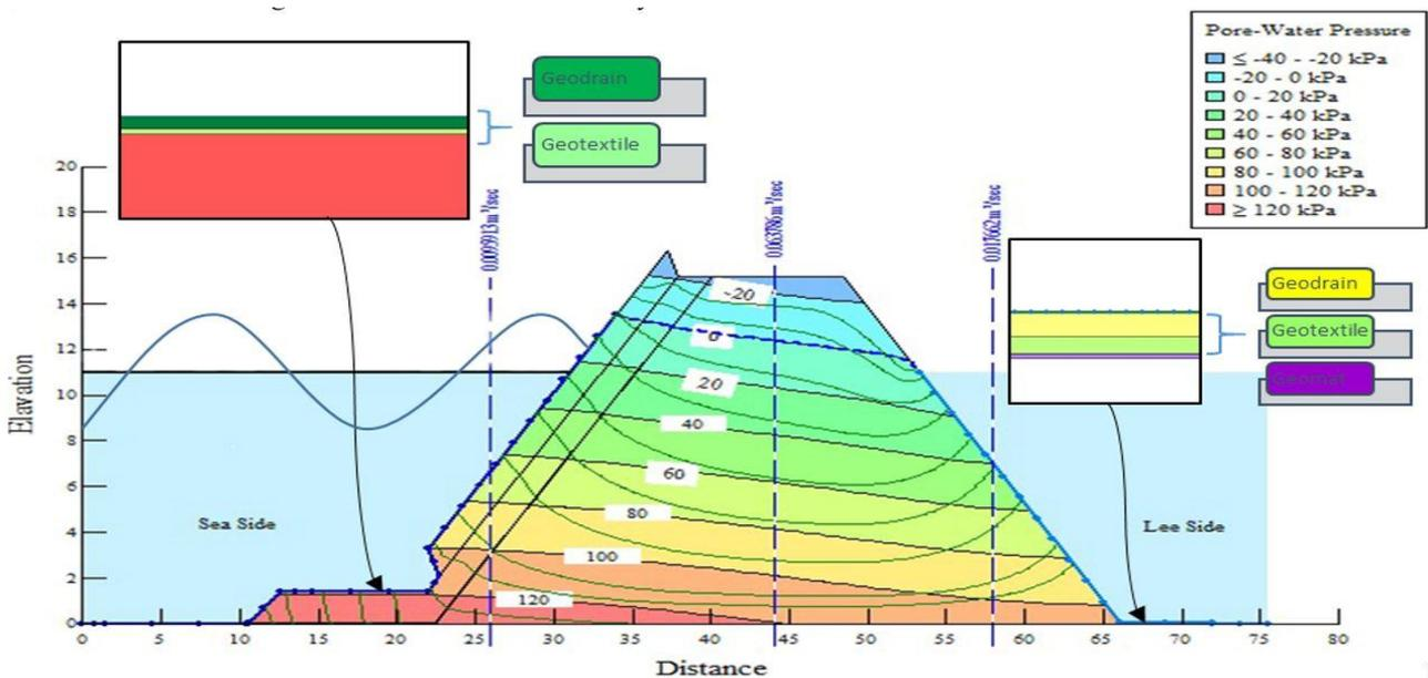
**Figure 20.** The model obtained from the use of geotextile and geodrain as filter, armor and geomat as matress
