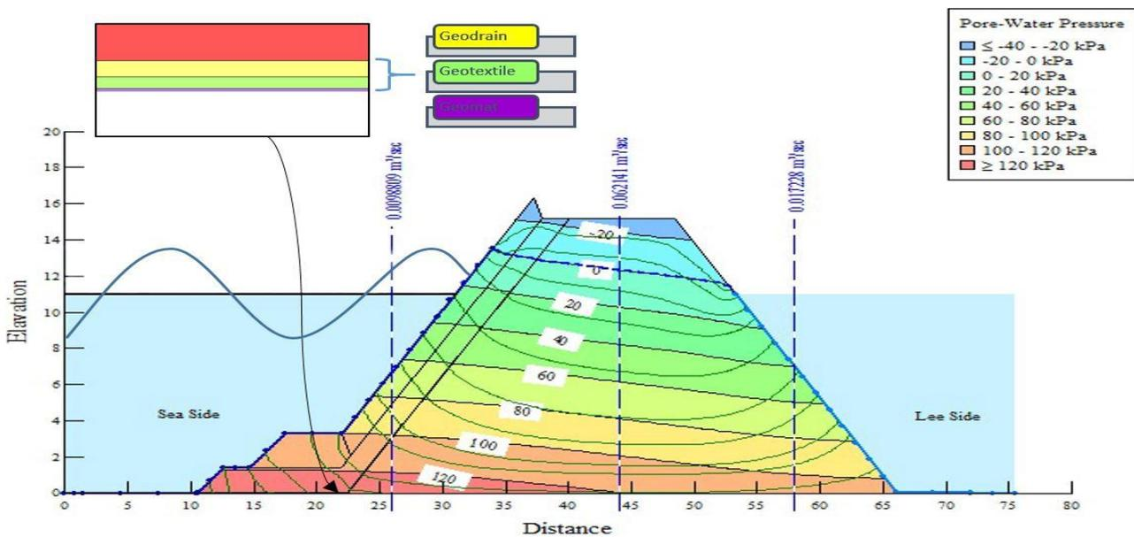
Figure 16. Use of geotextile and geodrain as filter layer and geomat as matress
