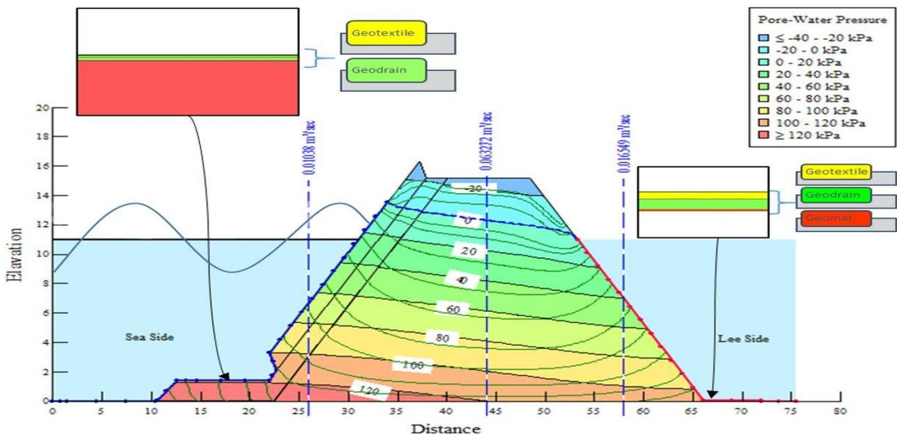
Figure 18. The model obtained from the use of geodrain and geotextile in filter and armor and geomat in matress
