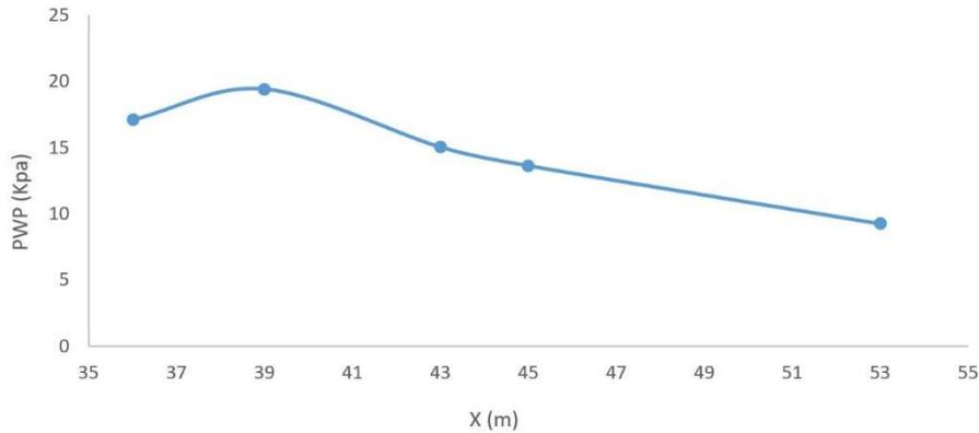
**Figure 5.** The pore pressure curve in in the primary breakwater
