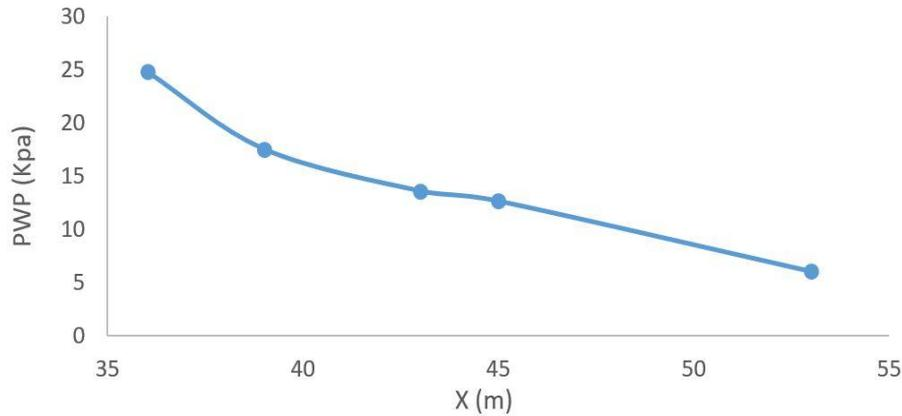
Figure 17. The pore pressure curve when using geotextile and geodrain as filter layer and geomat as matress
