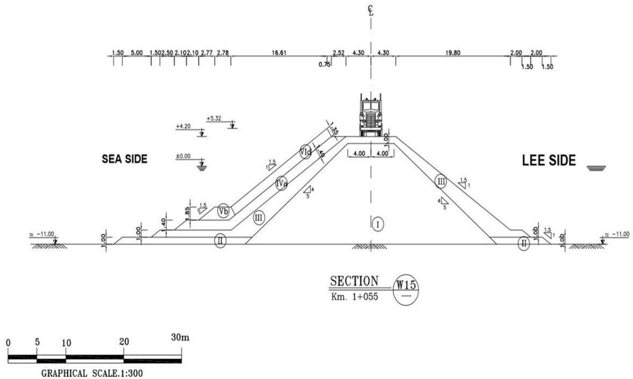
Figure 2. Section W15 West breakwater of Caspian port complex [16].
