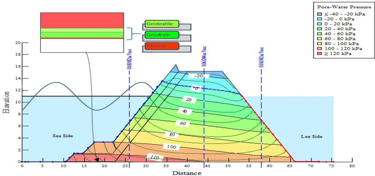
**Figure 14.** Use of geodrain and geotextile as filter layer and geomat as matress
