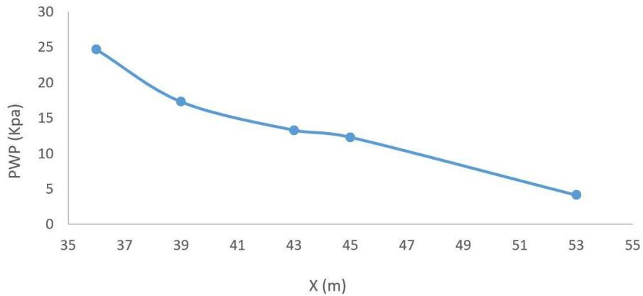
Figure 15. The pore pressure curve when using geodrain and geotextile as filter layer and geomat as matress
