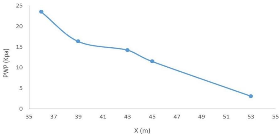
**Figure 9.** The pore pressure curve when using Geodrain and Geotextile
