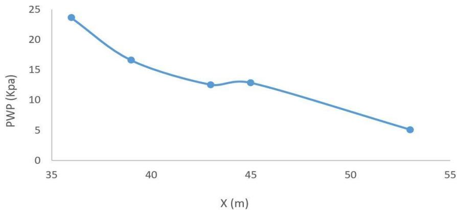
Figure 13. The pore pressure curve when using geotextile and geodrain as secondary armor and filter layer
