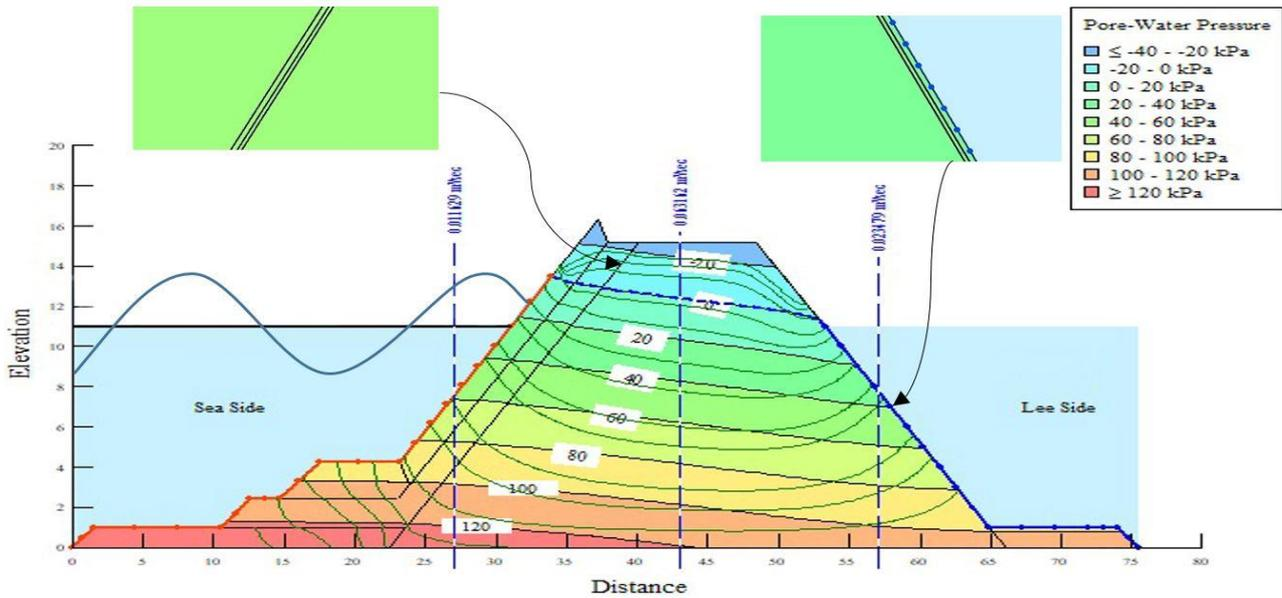
Figure 6. Use of geotextile and geodrain as filter layer
