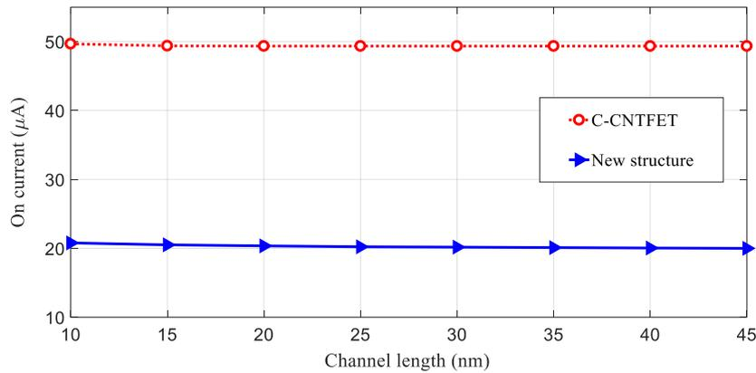
Figure 5. Saturation current variation by channel length while the bias is fixed at  $V_{GS} = 0.8\text{ V}$ ,  $V_{DS} = 0.8\text{ V}$ .
