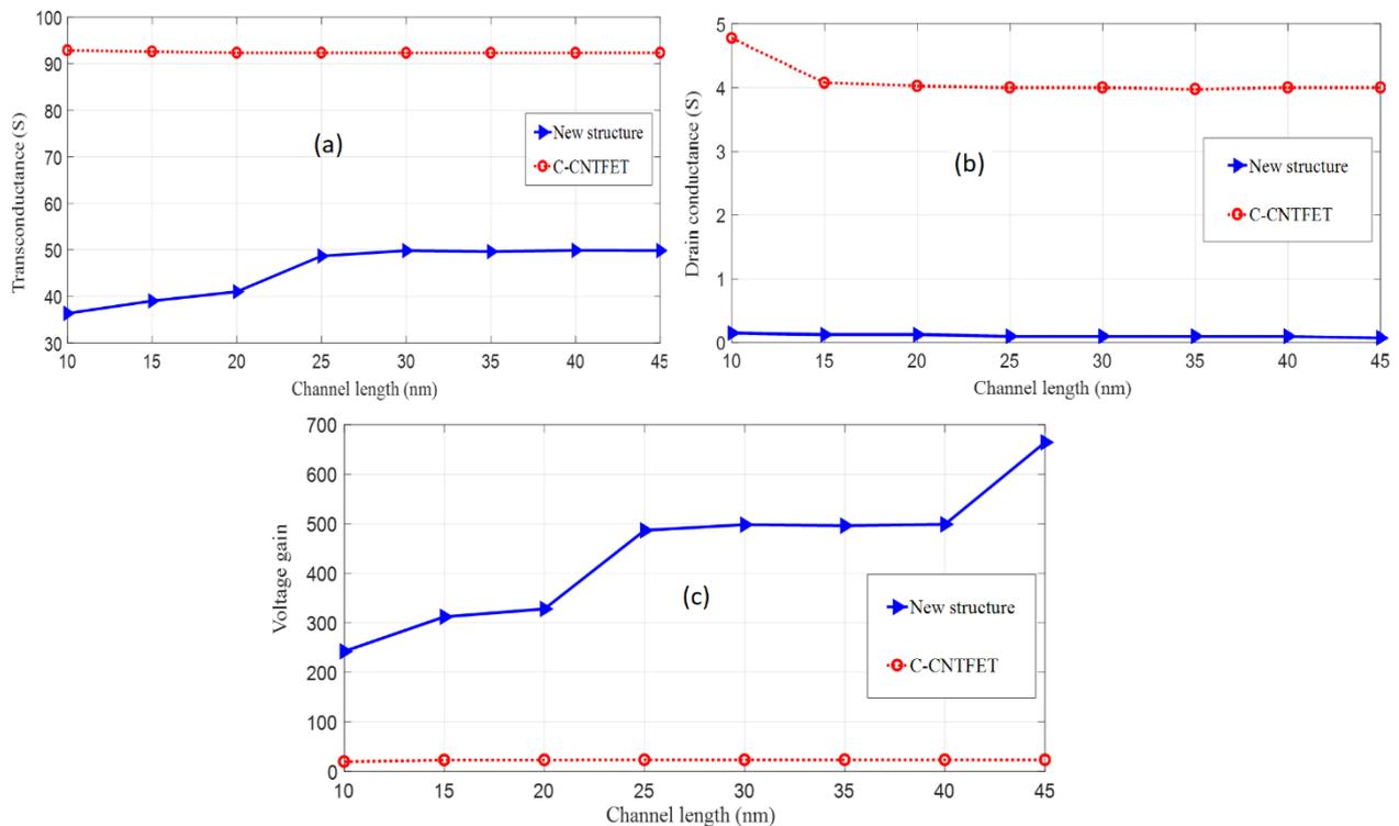
Figure 9. (a) Transconductance (b) drain- conductance and (c) the voltage gain diagram in terms of channel length for new structure and C-CNTFET
