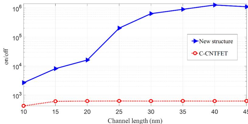
Figure 7. ON/OFF current ratio variations by channel length while the bias is fixed at  $V_{DS} = 0.8\text{ V}$ .
