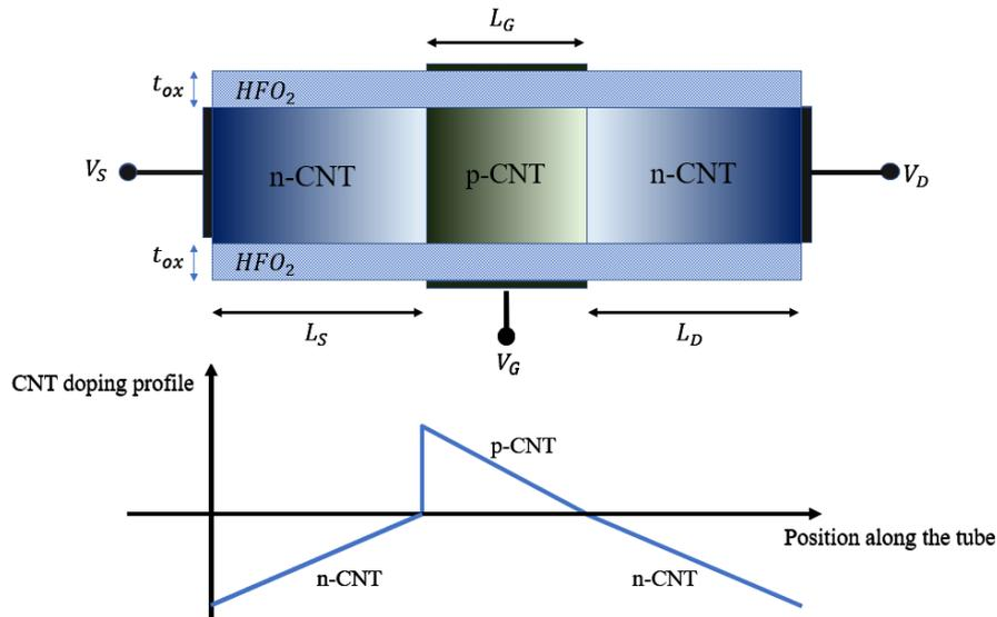
Figure 1. New structure of CNTFET at the doping distribution at each region to manage the BTBT.
