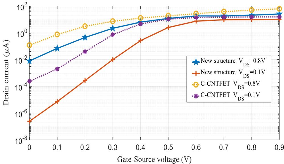
**Figure 3.**  $I_D$  diagram versus GS voltage for new and C-CNTFET structures at  $V_{DS} = 0.1$ , and  $0.8$  V and  $L_G = 10$  nm.
