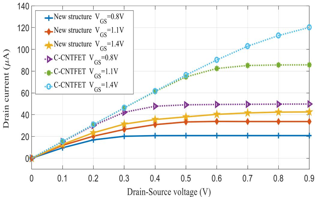
Figure 2. I<sub>D</sub> versus V<sub>D</sub> in terms V<sub>GS</sub> = 0.8, 1.1, and 1.4 V where L<sub>G</sub> = 10 nm for new and conventional devices
