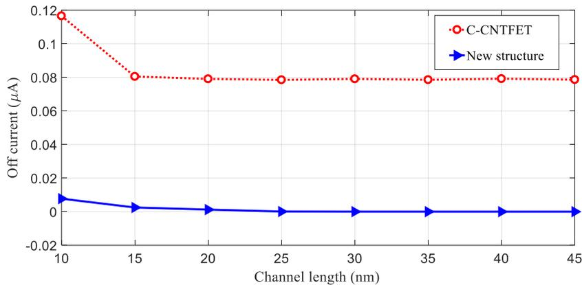
Figure 6. Leakage current variation by channel length while the bias is fixed at  $V_{GS} = 0.0\text{ V}$ ,  $V_{DS} = 0.8\text{ V}$ .
