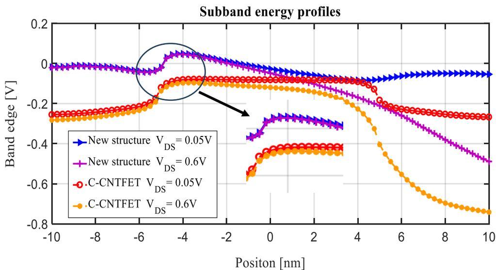
**Figure 4.** Diagram of potential distribution along the nanotube length for new structure and C-CNTFET at  $V_{DS} = 0.05, 0.6$  V And  $V_{GS} = 0.5$  V.
