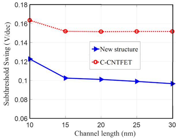
Figure 8. The SS diagram in terms of channel length for the new structure and C-CNTFET
