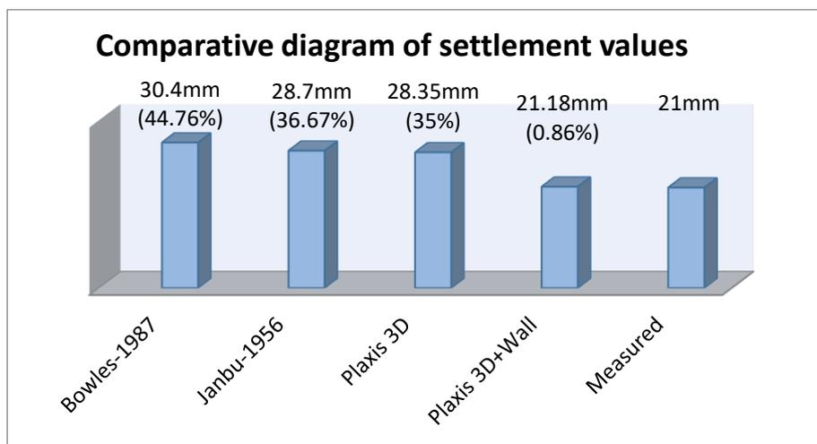
**Figure 8.** Comparative diagram of settlement values
