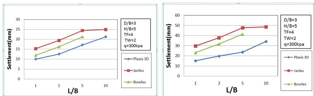
**Figure 9.** Effect of foundation length for soil types 1 and 2
