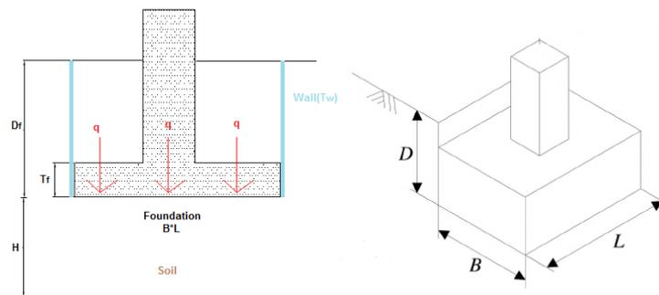
**Figure 3.** Studied Geometric parameters
