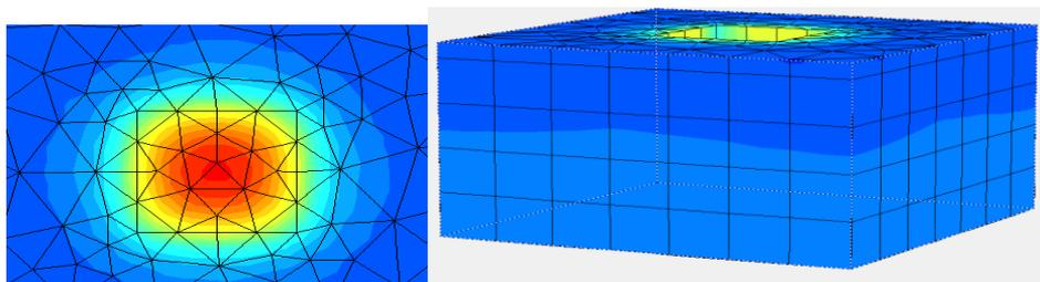
**Figure 5.** Image of Plaxis 3D Foundation output of model without wall
