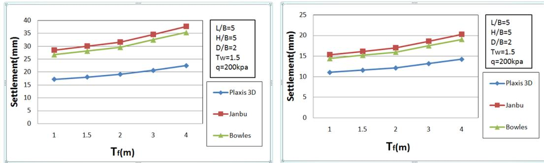
Figure 12. Effect of foundation thickness for soil types 1 and 2
