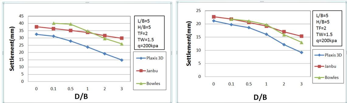
*Figure 10.* Effect of foundation depth for soil types 1 and 2
