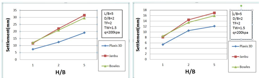
*Figure 11.* Effect of soil depth for soil types 1 and 2
