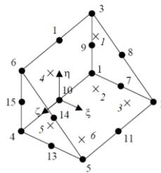
**Figure 2 .** Volumetric element used in Plaxis program
