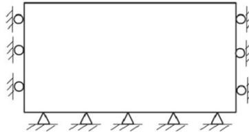
**Figure 4.** Model boundary conditions
