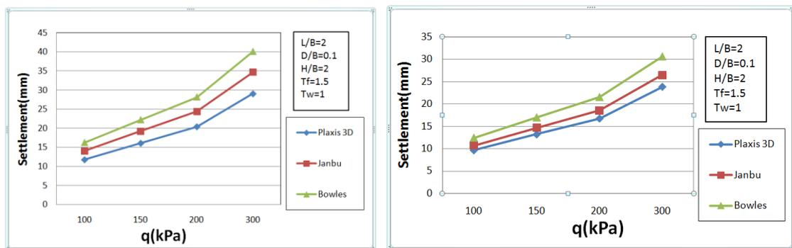
Figure 13. Effect of load change for soil types 1 and 2
