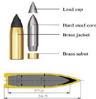
Figure 3. Geometry and dimensions of the AMP2 projectile
