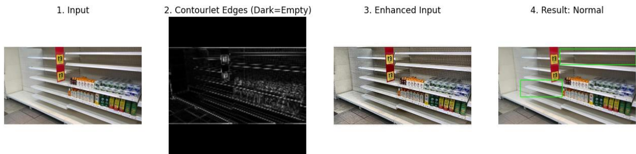
Figure 11. Output error of the system for an OOS shelf sample, where despite an incorrect final shelf classification, empty spaces are partially detected.
