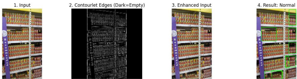
Figure 6. System output for a normal shelf example, showing accurate detection of empty or reduced spaces and correct identification of the overall shelf status as normal.
