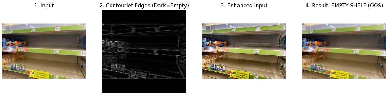
Figure 9. System output for an empty shelf (OOS) example, demonstrating accurate detection of shelf emptiness and correct triggering of the OOS alert.
