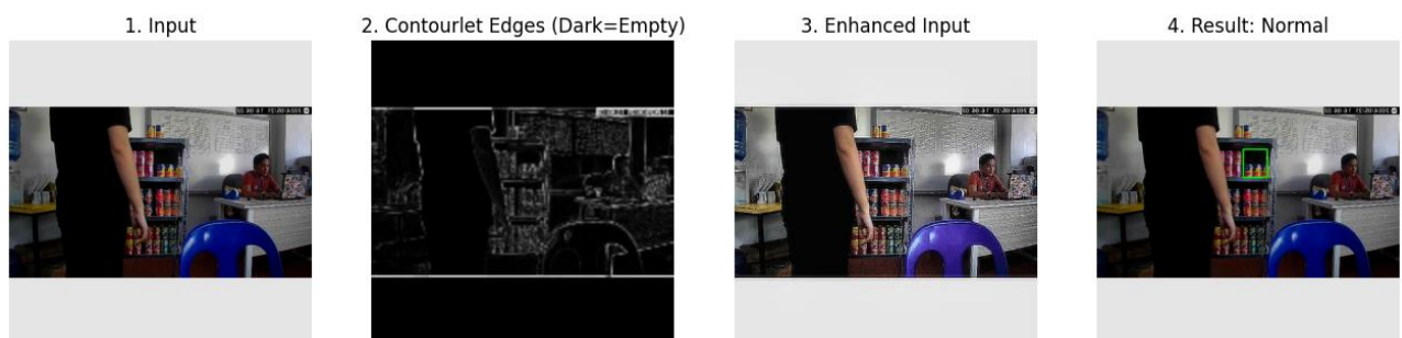
Figure 8. System performance under occlusion: Accurate detection of reduced spaces and normal shelf status despite partial human obstruction.
