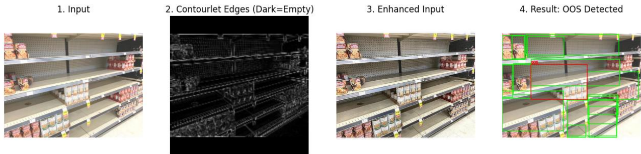
Figure 10. System output for a partially empty shelf (OOS) example, showing near-accurate identification of empty and reduced spaces and correct classification of the overall shelf status as OOS.
